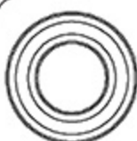
Bearing 軸承 (φ 12x φ 24x6mm) x 3
