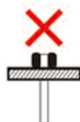
Too much solder may cause false welding which looks like beehive-shape on surface. 焊錫太多表面呈蜂窩狀的假焊
