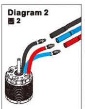
The motor rotates in different direction with different brand ESCs. If the wrong rotating direction happens, there are two ways to adjust it:
