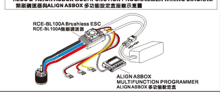
Apply another three-pin wire (with JR male connectors at both ends for connecting ESC and Multifunction Programmer. Plug the three-pin wire into ESC "-+P" port, and also plug into multifunction programmer "ESC" port.
