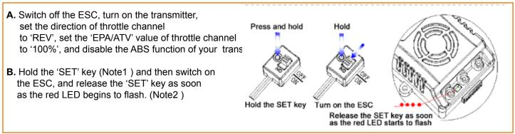
Note 1: The 'SET' key of S18 is beside the main switch of the controller.
