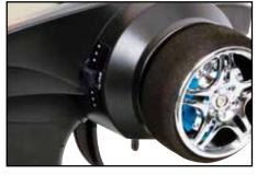
**Throttle Trim:** Trim the throttle servo slightly when the trigger is at the neutral position.
